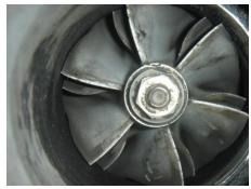
Compressor wheel damage is caused by dust entry into the compressor housing air entry area of the turbocharger.
